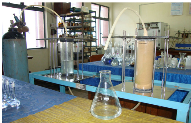
Fig. 1 Column experiment for removal of pollutants from AMD
